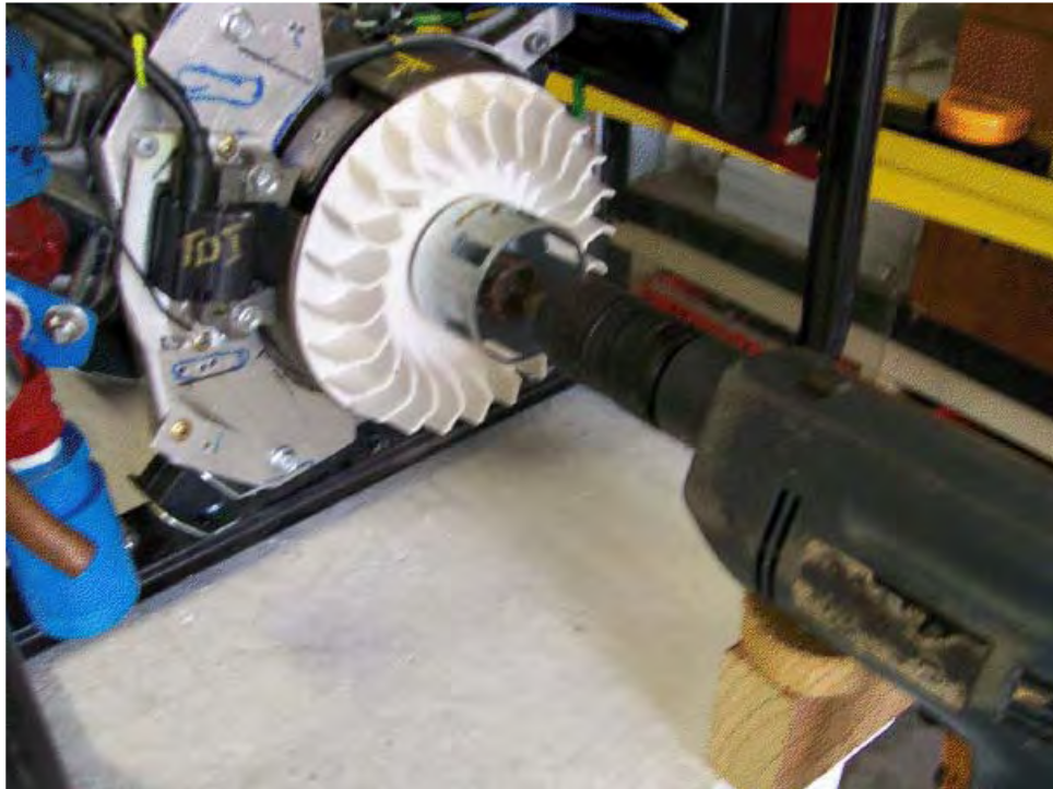
Figure 80: Photograph of Selwyn's latest generator conversion having it's new spark timing checked out.
