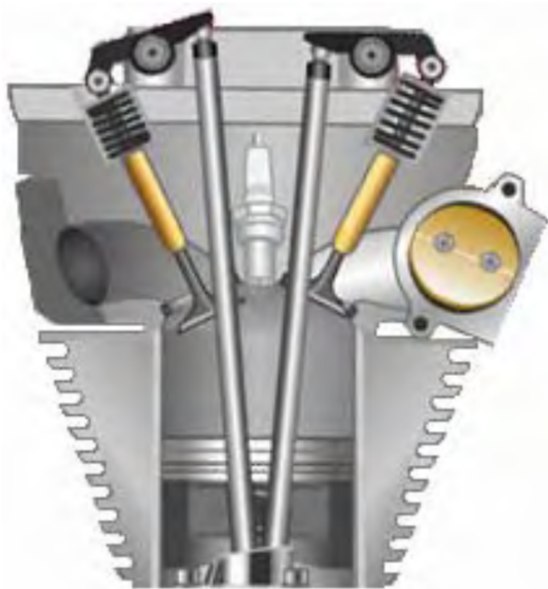
Figure 56: Suppressing the additional “waste” spark. So, this leaves us with two engine adjustments: timing delay and waste spark elimination. There is a technique which can be used with many engines and which deals with both issues at the same time. Most engines of this type are four-stroke engines with intake and exhaust valves, perhaps something like this.
