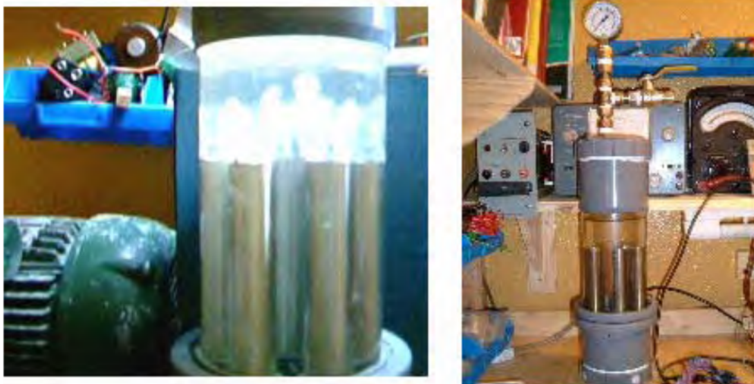
Figure 5: Dave Lawton's electrolyser with acrylic tube section to allow the electrolysis to be observed.
