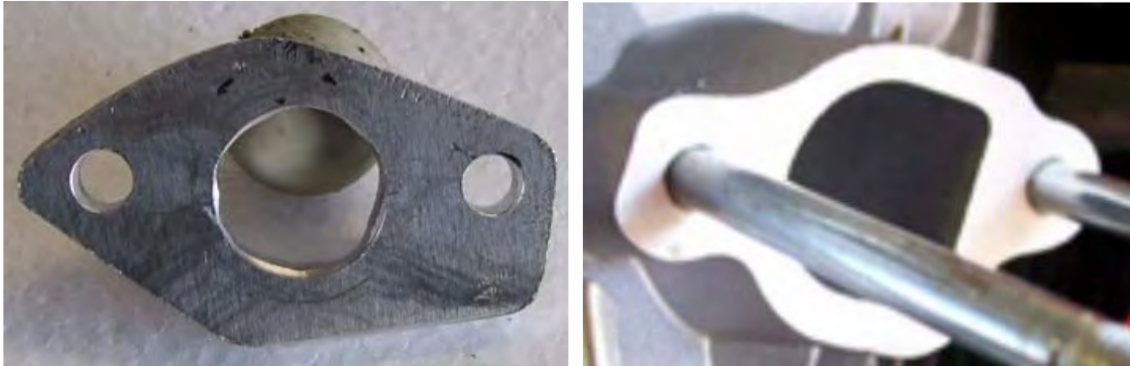
Figure 71: A piece of 1/4" (6 mm) thick aluminium plate, cut and shaped to the size of the carburettor gasket. The edges are then filed to create a fit on the engine port.
