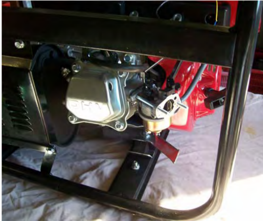
Figure 63: Fuel tank to be removed in GX4000i generator, held in place with four bolts.
