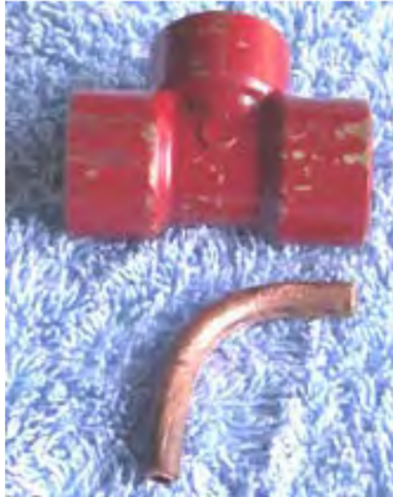
Figure 81: Selwyn's construction of a Venturi tube. A short length of 1/4" (5 or 6 mm) diameter copper tubing is used.
