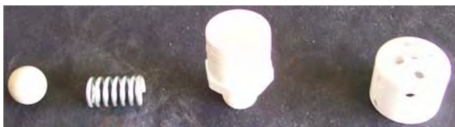
Figure 66: The PVC plastic fittings: 1/2" to 1-1/4" reducer and a 1-1/4" End Cap, along with the roller ball from an old-fashioned mouse and a relatively weak compression spring.
