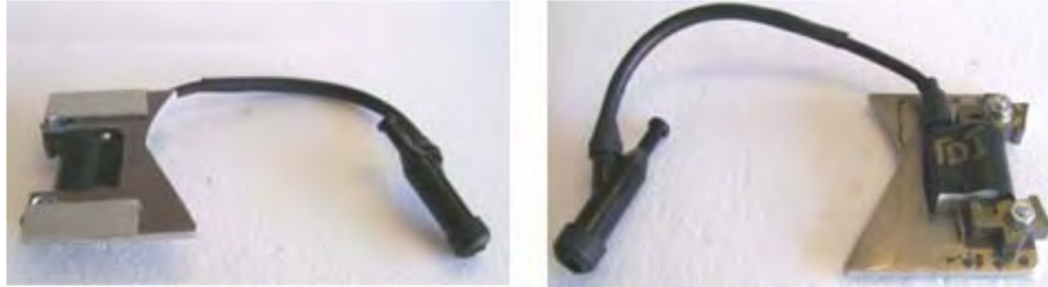
Figure 76: Selwyn's aluminium TDI adaptor plate which he made from 2 mm thick aluminium sheet.
