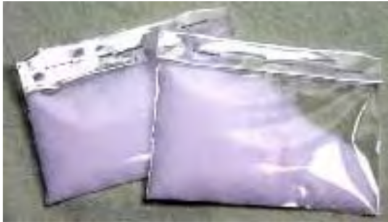
Figure 86: Treating and cleaning the Hogg electrolyser using add 1 packet of citric acid, shown in the photograph, for each 3 litres of water used to fill the electrolyser.
