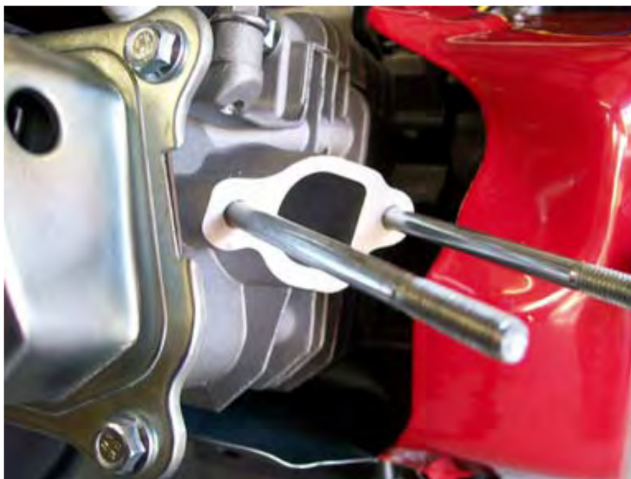
Figure 64: Once the fuel tank is removed in the GX4000i generator, it allows access to the carburettor, which must also be removed as it is not used. See comparison of this figure and figure 63.
