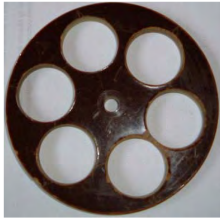
Figure 7: The mounting rings for the tubes made from a suitable plastic, i.e. a chopping board.
