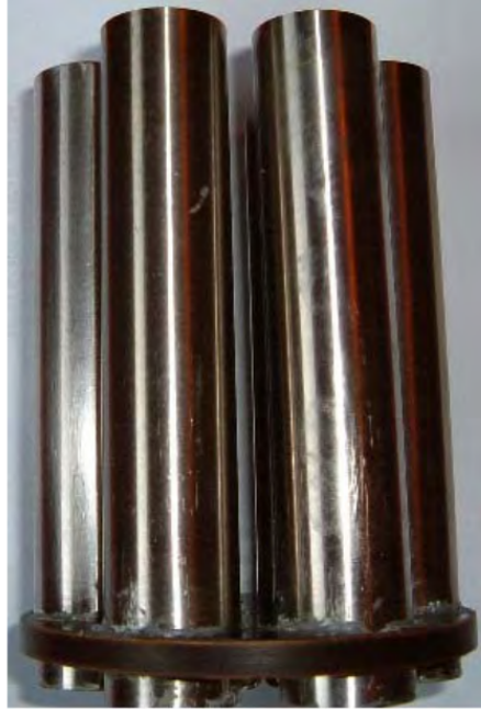
Figure 8: 316L grade stainless steel, seamless tubes.
