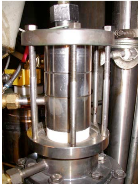
Figure 2.6. Photograph of plasmatron fuel reformer used for experiments with propane, natural gas, gasoline and bio fuels during the last year of the program (gen 3a)
