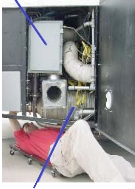
Figure 4.15 Picture of part of plasmatron diesel reformer system in the back of the bus
