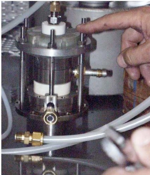
Figure 4.2. Compact low power plasmatron fuel converter used for these tests
