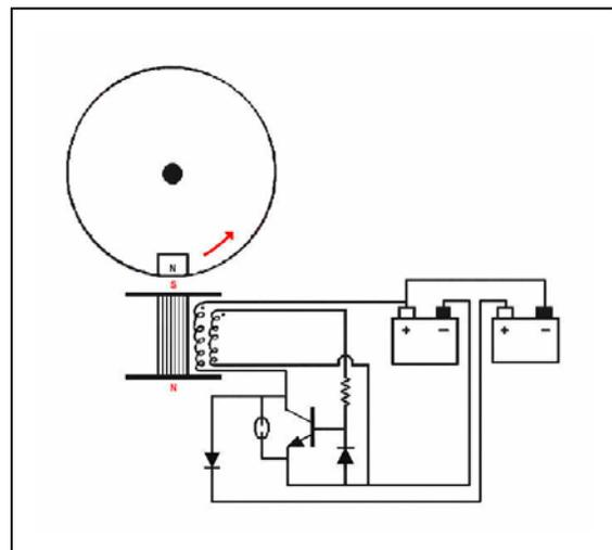
The attraction of the magnet to the coil has produced some momentum on the wheel, so it slips past the top of the coil.
