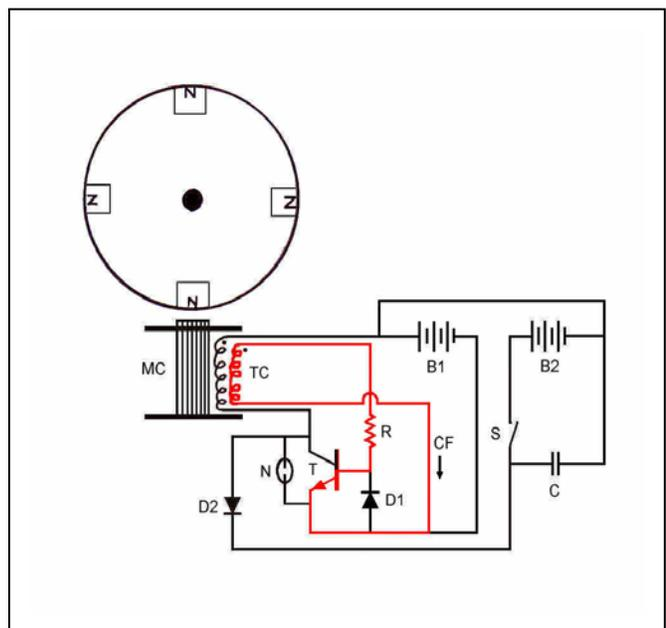
The **Output Section** of the circuit is next. After the Transistor (T) turns OFF, the current supplied by Battery (B1) stops supporting the magnetic field in the Main Coil (MC). When this happens, the magnetic field must collapse. In doing so, it induces a burst of electrical energy in Main Coil (MC) that can be collected. Capturing this energy is one of the main reasons for learning about this project.
