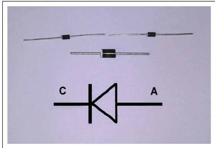
Diodes usually appear as a small cylinder with a wire coming out of each end. Diodes will usually show the symbol, or a single stripe at one end of the cylinder, as the examples in the picture shows. One end of the diode is called the "Cathode" (C) and the other end is called the "Anode" (A). Electricity will flow through the device when the Cathode is "more negative" than the Anode, OR if the Anode is "more positive" than the Cathode. The stripe indicates the Cathode end of the Diode.
