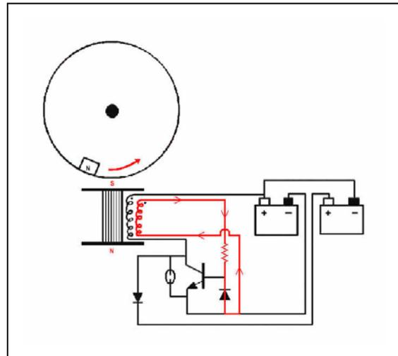
When the magnet is directly over the top of the coil, the permanent magnet has induced its field into the coil core as much as it can. At this point, the "change in magnetic flux" that was inducing the current in the Trigger Winding stops rising, and so the current in the Trigger Coil also stops flowing.
