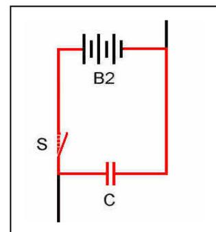
Of course, the final Output is for the Capacitor (C) to discharge into Battery (B2), as shown when Switch (S) closes temporarily. In this section, Capacitor (C) is the power source, Switch (S) is the control device, and the charging of Battery (B2) is the end result, the final Output, and the last operation of the circuit.
