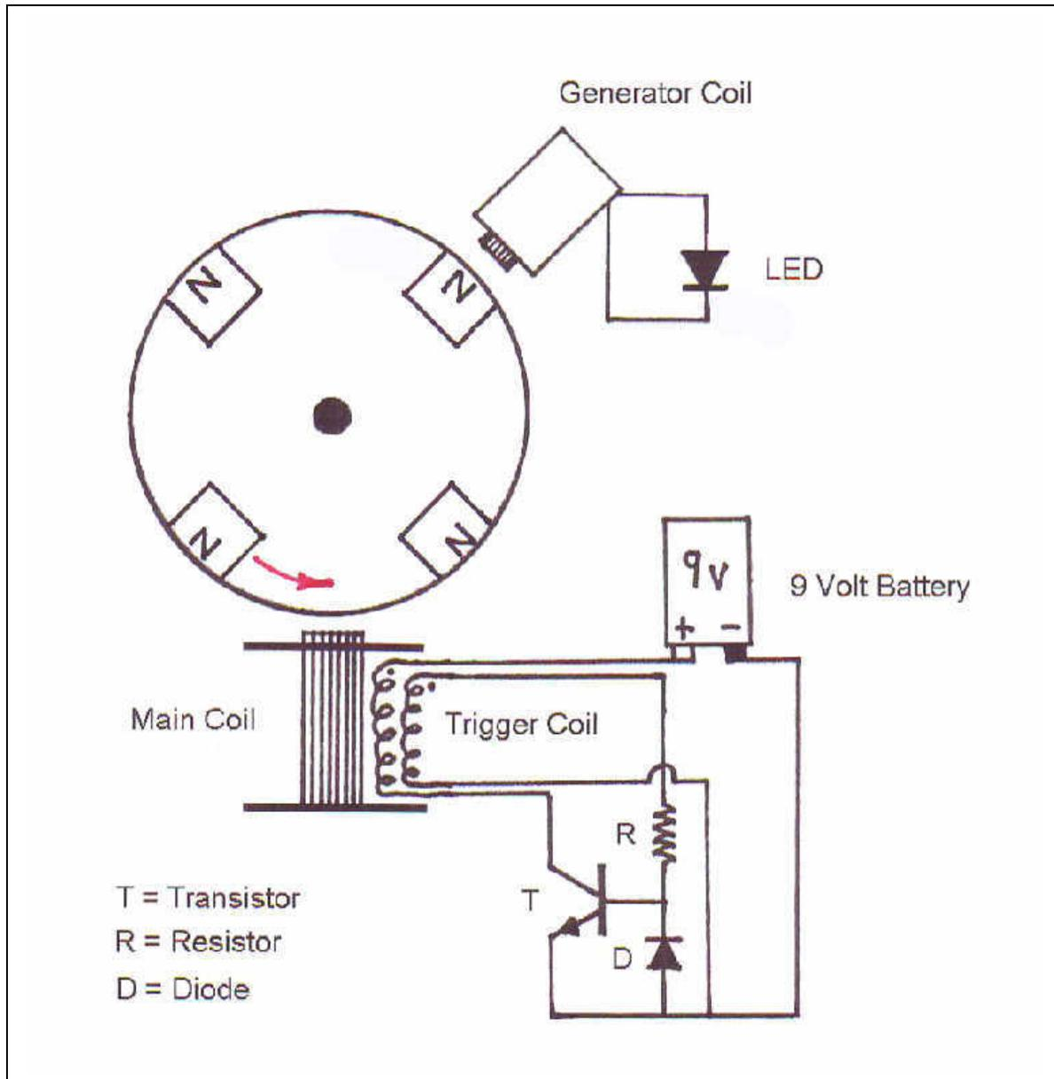
The Main Coil has some iron rods in the center of its structure and they participate in getting the process started. As one of the magnets on the wheel approaches the iron core of the Main Coil, it becomes attracted to the iron and so, it moves in the direction of the **RED ARROW**.
