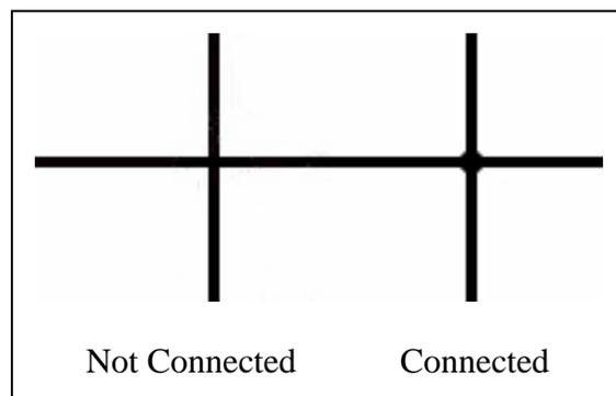
The second method is used in some of the patents in the back of the book and looks like this. The image on the left, where the lines cross, represents where two wires cross over each other in the diagram, but ARE NOT electrically connected. The image on the right, where the lines cross with a
