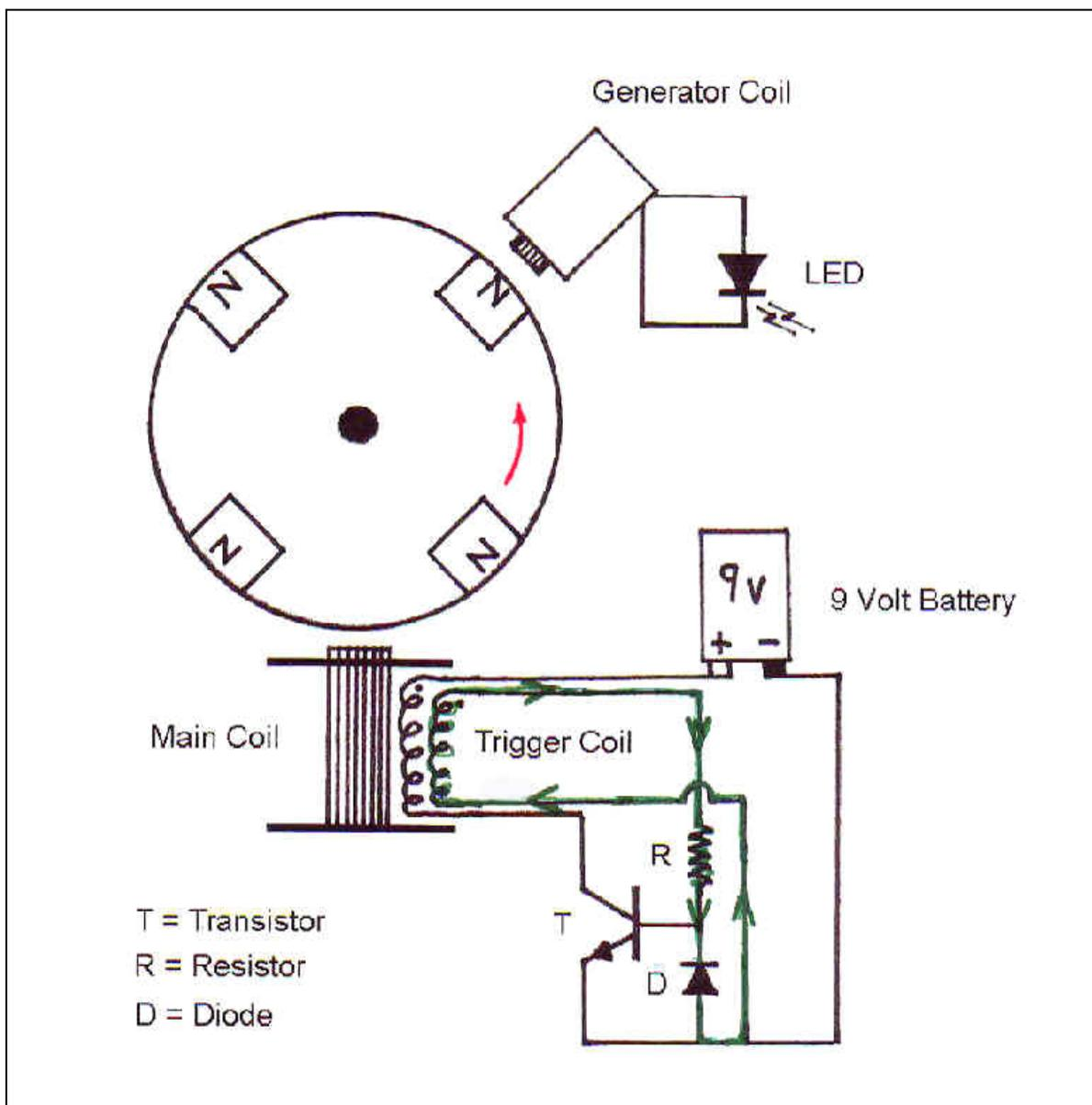
Meanwhile, the other magnet is approaching the generator coil, and is also being attracted to the small amount of iron there. As that magnet slips past the generator coil, a current is induced that lights up the LED for a single flash. As the rotor speeds up and these flashes happen more often, the LED appears to be ON all of the time.
