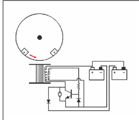
As the magnet approaches the coil, it starts to magnetize the iron core and this "change in magnetic flux" begins to induce a current in the Trigger Winding in the direction of the **RED ARROWS**. Since this current is in the wrong direction to activate the Transistor, the Transistor stays OFF, and no power is used from the Battery while the magnet approaches the coil.
