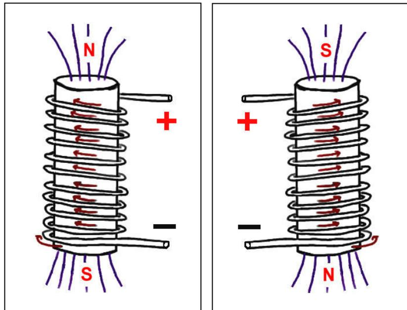
winding produces a North Pole at the top and a South Pole at the bottom.
