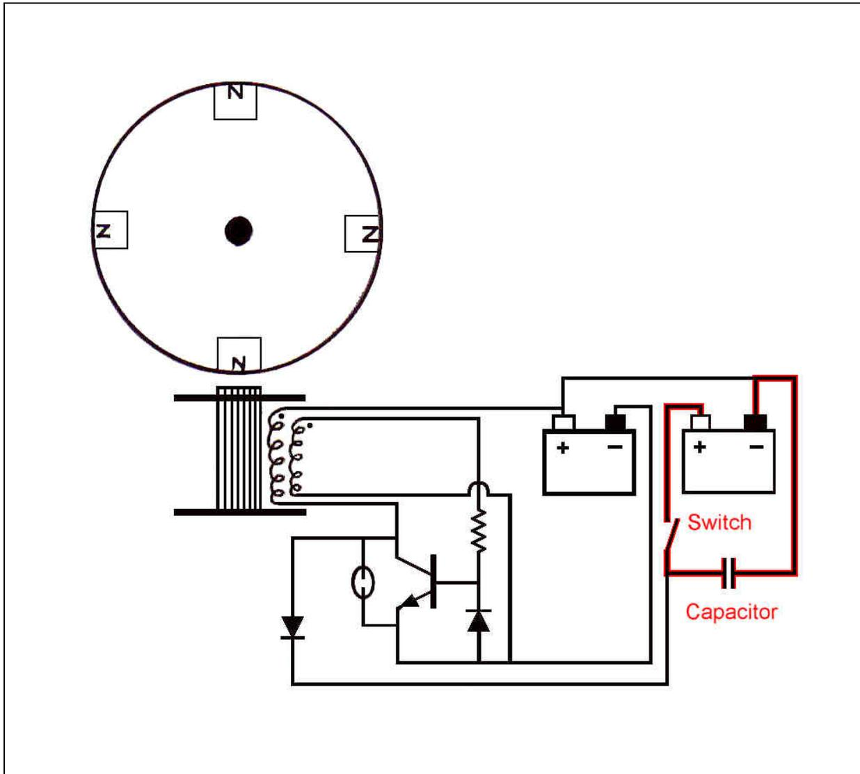
Here, we ADD a capacitor and a switch. Now, the voltage spikes from the Main Coil can be collected in the capacitor when the switch is open and periodically delivered to the battery when the switch is temporarily closed.
