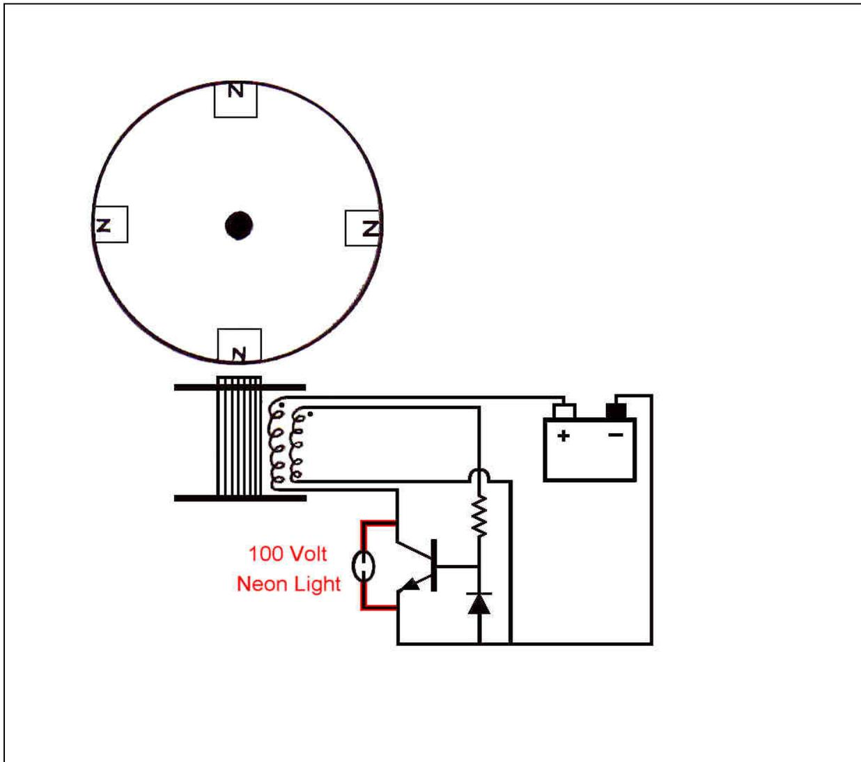
As you can see, the NEON LIGHT is placed directly across the output terminals of the transistor that is turning the coil ON and OFF from the battery. This way, when the transistor turns OFF, the voltage spike can create a temporary pathway back to the battery AFTER the voltage rises high enough to turn the NEON LIGHT ON. Otherwise, when the Neon Light is OFF, no circuit connection is being made.
