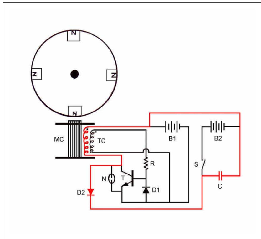
Diode (D2) is the control component in this section of the circuit. It allows the discharge of the energy in Main Coil (MC) to divert around the Transistor (T) and also facilitates the charge in Capacitor (C) to build up without discharging. The charging of Capacitor (C) is the desired, end result of this section of the circuit.
