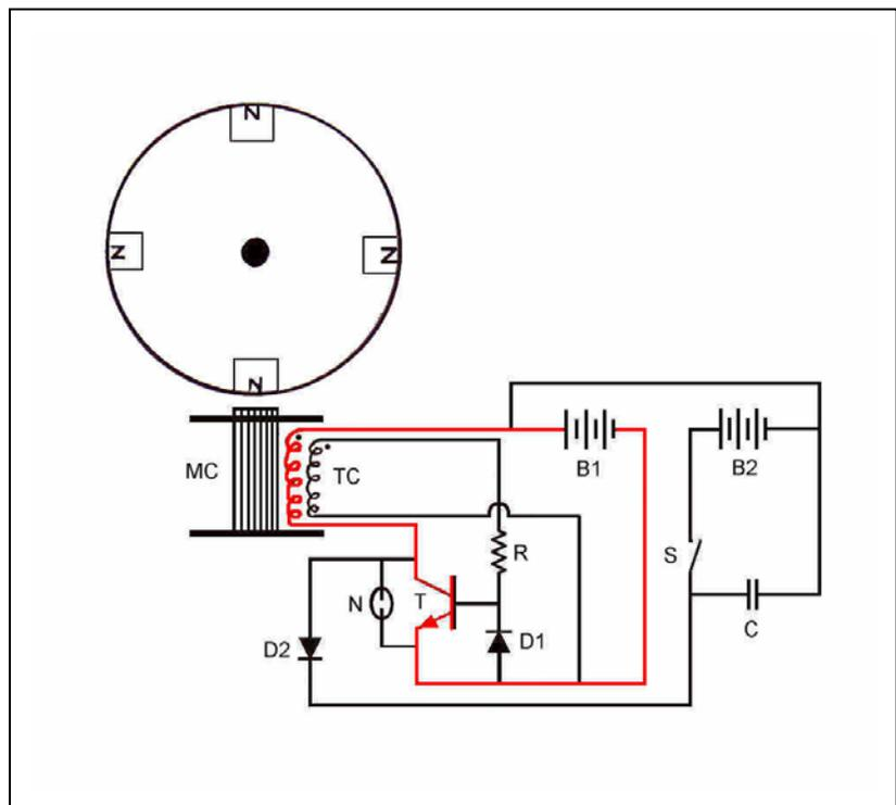
This is the power section of the circuit for this project. When this function happens, the Main Coil (MC) is being magnetized, and the magnet on the rotor wheel is being pushed away. It is the only time when electricity is coming out of Battery (B1) and the only time when the system is consuming any energy that counts as an "input."
