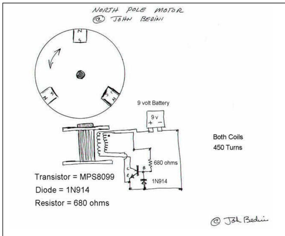
The only differences between his first drawing, shown above, and Shawnee's project were that Shawnee's rotor wheel had four magnets on it, and there was an extra generator coil mounted on the top that lit the LED.
