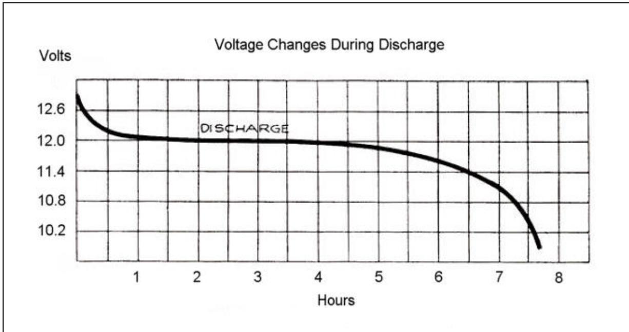
As you can see from the graph, as soon as a load is connected to the battery, its voltage drops a little. Then the voltage stabilizes and remains constant for a long time before dropping off more at the end.
