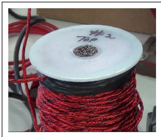
So, here is a close-up photo of the "top" of the coil. This makes a coil that is wound in the "counter-clockwise" direction. When you get this far, you should be really proud of yourself! You have finished "making" the coil!
