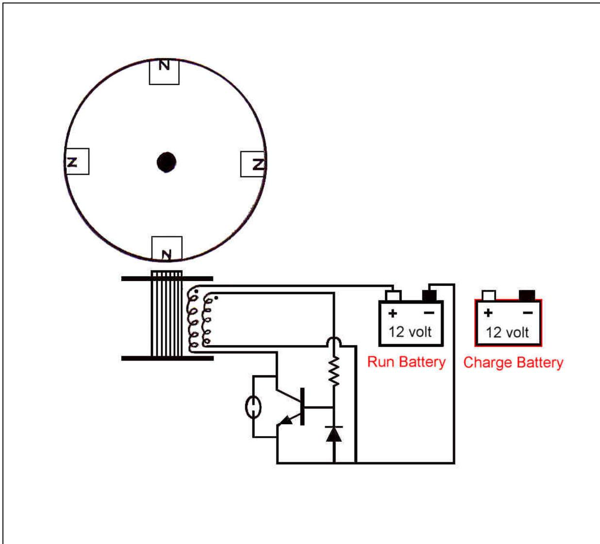
By adding a second battery to the circuit, one battery can now Run the system and the second battery can now be CHARGED by the system at the same time. This allows both batteries to operate at their highest levels of efficiency.
