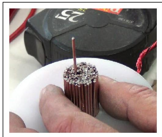
It's important that all of the rods are cut to the same length so that they all come through to an equal height on the "other end" of the coil, which is going to be the "top" of the coil that faces the magnets on the wheel.
