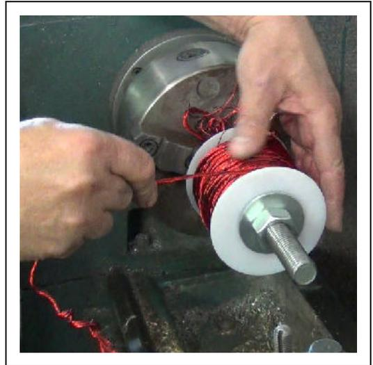
While still holding the cable, John applies some "super-glue" to the last windings, where the cable will be coming out of the coil.
