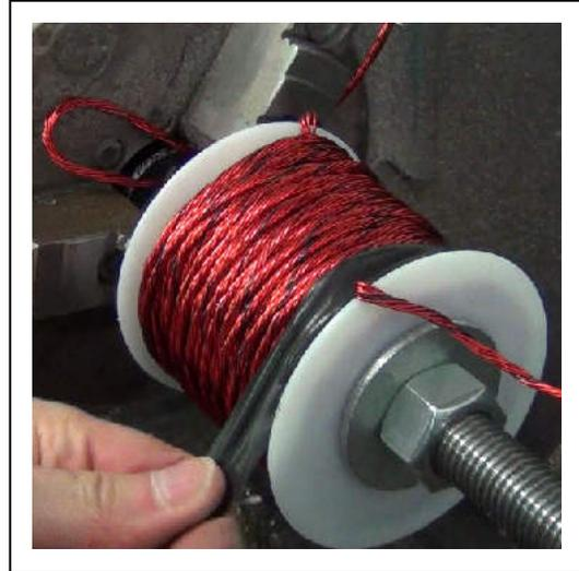
At this point, the coil is removed from the lathe and the bolt is removed from the center of the spool.
