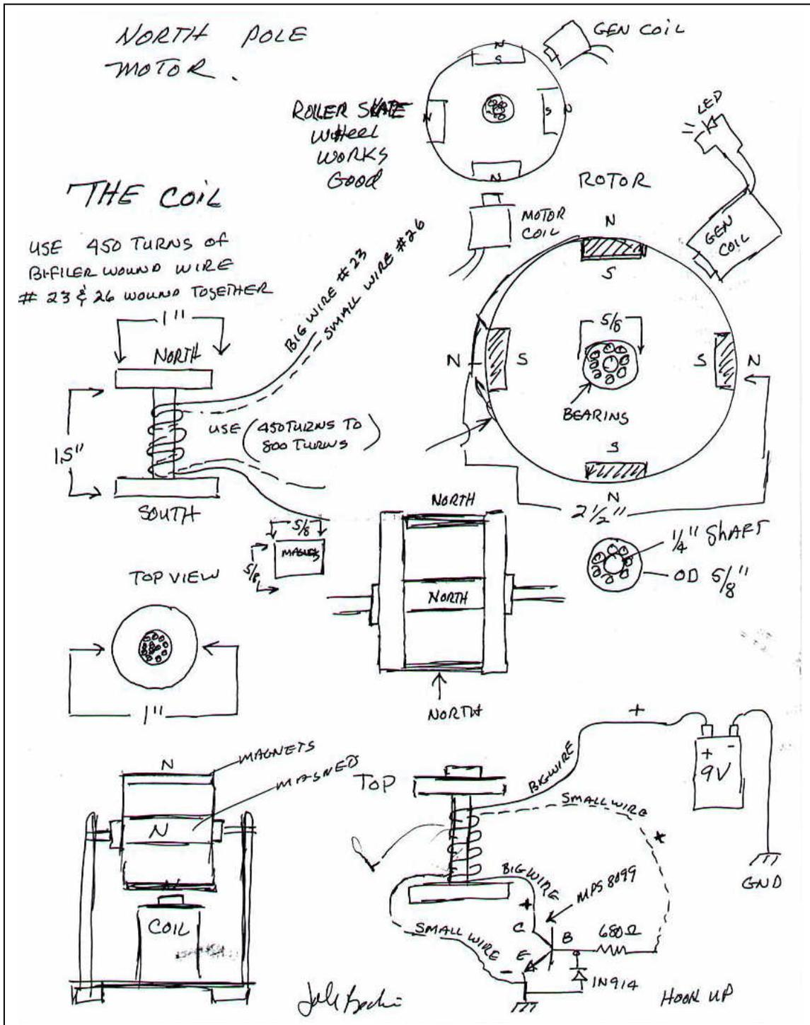
As you can see, this is a fairly simple little project. It can be built using a little frame to hold a roller skate wheel that has 4 small permanent magnets glued onto it. It also has two small coils of wire, a 9 volt battery and four electronic components: a MPS8099 transistor, a 1N914 diode, a 680 ohm resistor and an LED. The question is, what is so special about this device that a 10 year old could win a school Science Fair with it?
