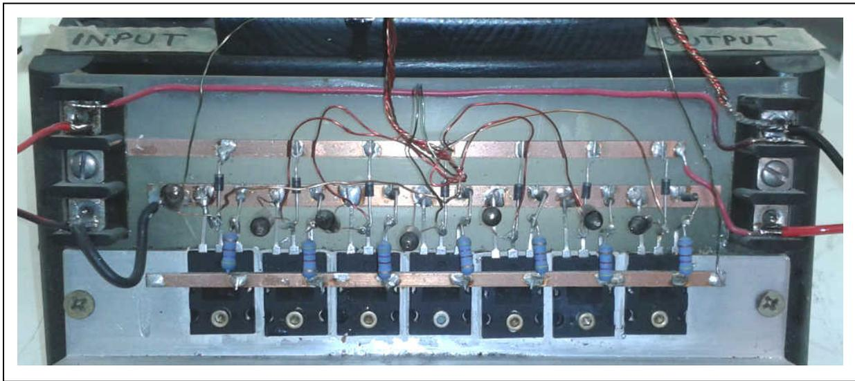
What you are looking at in the photo above is 7 circuits like the diagram to the right, where for each of the Main Coil wires there is a transistor, a neon bulb, a resistor, and two diodes. The wires going to the Run Battery are on the terminal block on the left side, labeled INPUT. The **RED** wire goes to the battery Positive and the **BLACK** wire goes to the battery Negative.
