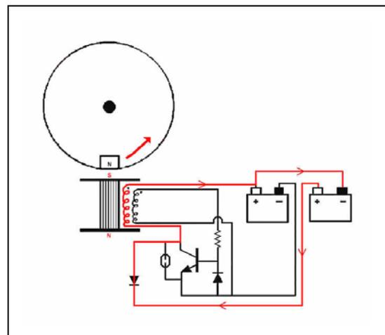
With the collapse of the magnetic field in the Main Coil, the North Pole of the magnet on the wheel is attracted to the coil much less, and so it proceeds out of the field with all of the stored momentum it accumulated during the attraction period.
