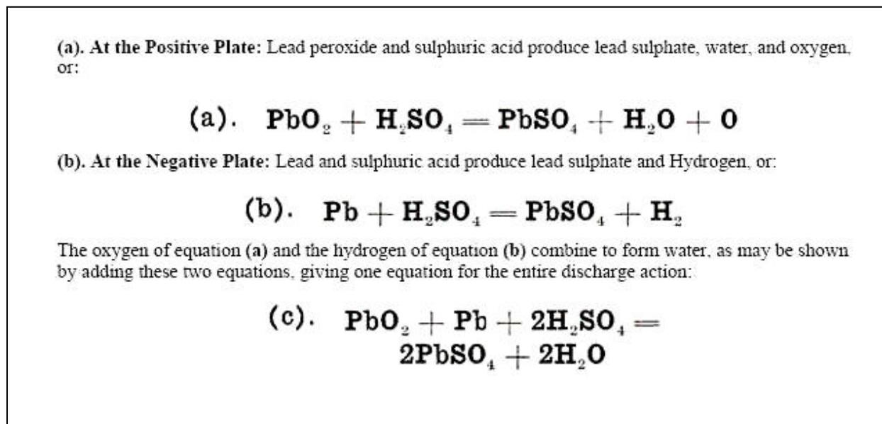
So, what happens when electricity is taken out of a battery? The answer is expressed above in equation (c). Two molecules of the acid in the electrolyte combine with the lead materials of the positive and negative plates to form two molecules of water and two molecules of lead sulfate.
