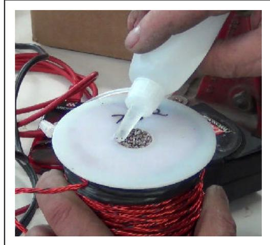
Next, apply "super-glue" around the edges of the rods and all across the surface of the rods, waiting a few minutes and then doing it again. You will see that some of the glue seeps all of the way down through the stack onto the cardboard. Make sure all of the rods are securely glued in place.
