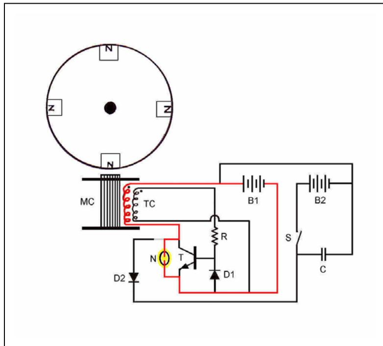
(MC) through Battery (B1). While this is not the preferred way to collect this energy, it does allow the energy to be safely dissipated without damaging Transistor (T) by subjecting it to a very high voltage spike.
