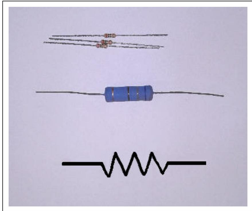
The three small resistors shown at the top of the picture are typical  $\frac{1}{4}$  watt resistors, used in many electronic devices. You may be able to see some colored stripes on them. These stripes represent a code which reveals the resistance value of the component.
