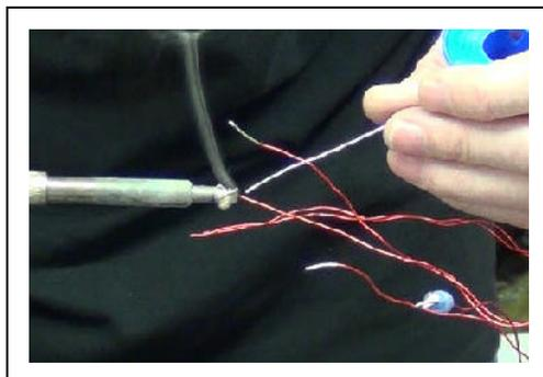
should not be done until the wires are cut to proper length during final assembly.
