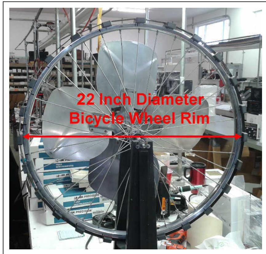
24 permanent magnets, measuring 1 x 2 x .5 inches, made from Ceramic #8 material, are mounted around the rim with a uniform 3 inch spacing between them. All magnets should have the NORTH POLE facing outward.
