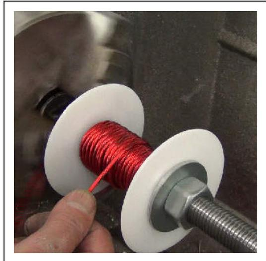
In the next photo, the coil has been wound to the end of the cable. John has purposefully ended the winding process with the cable at the outer end of the spool. This will be the "top" of the coil.
