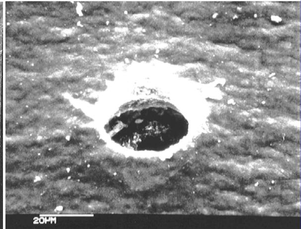
Fig. 13 Exit side of an EV strike on silicon carbide grain coated on a 0.001" thick aluminum foil.
