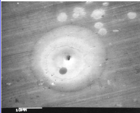
Fig. 1 EV strike on 6 micrometer thick aluminum foil.
