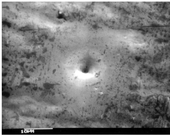
Fig. 2 EV strike on 6 micrometer thick aluminum foil.
