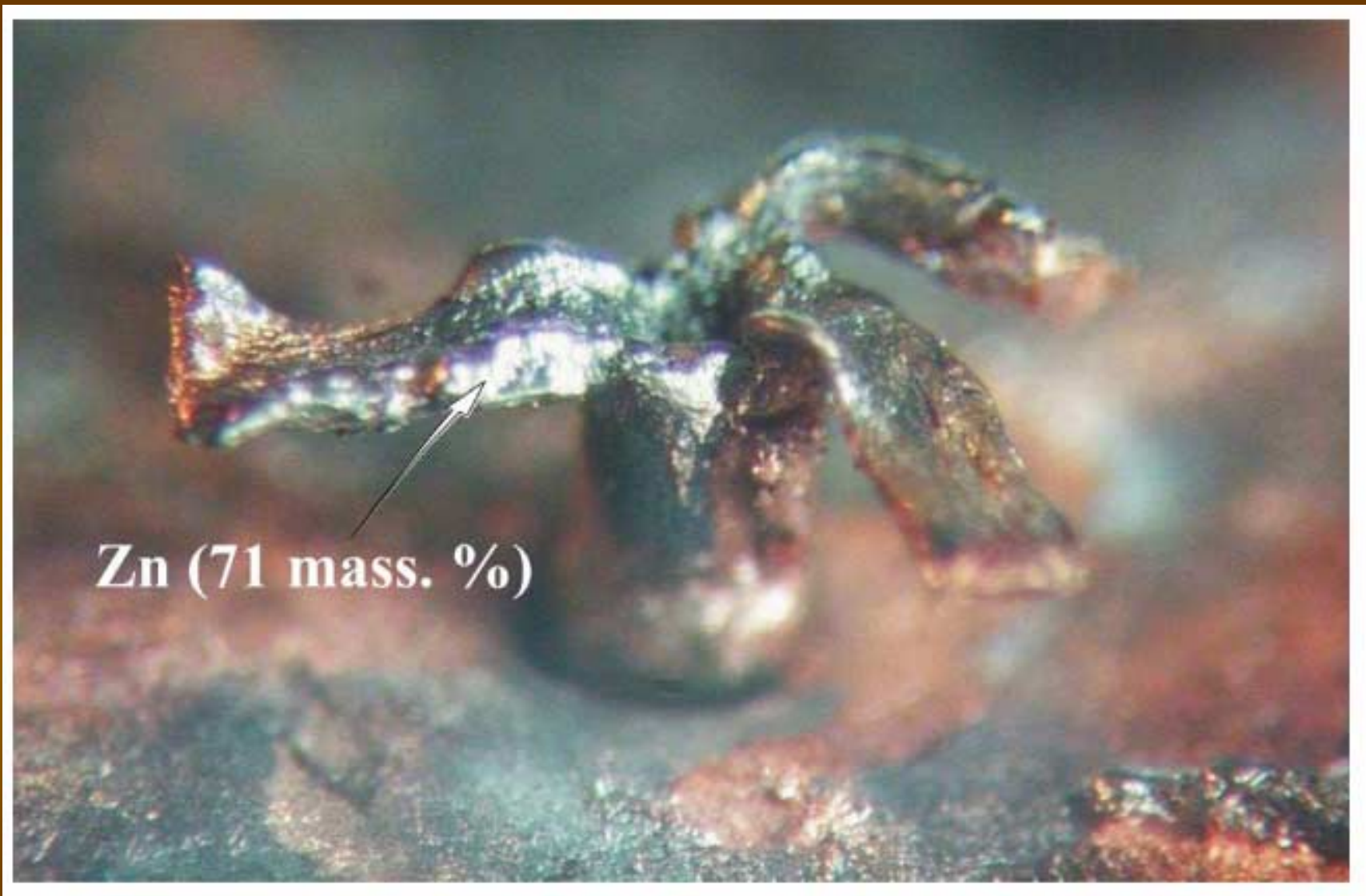
Copper target after the experiment, with traces of solidified silver-and-white “lava” on its “petals”, which had flowed out of the target center.
