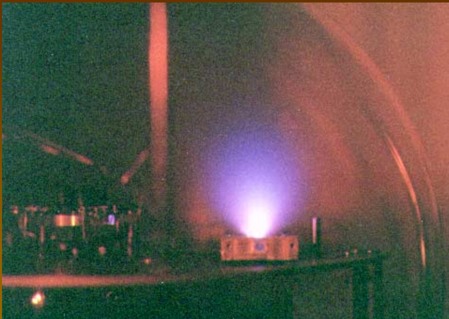
Fig. 8 Front view of plasma plume with cover removed
