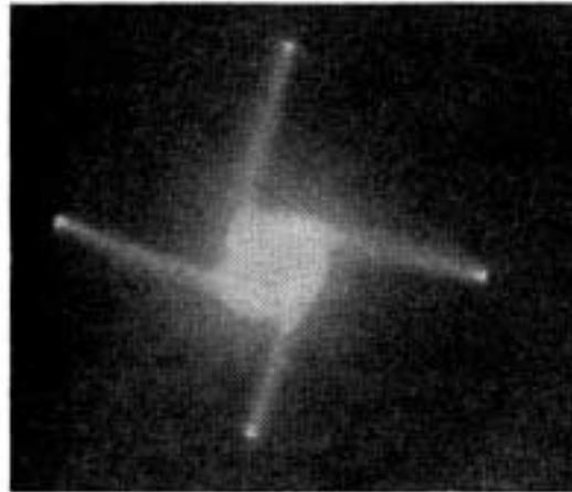
In both cases, the guns were purposely misaligned to show the attractive force between the plasma structures. With modern EVO guns, much better aiming is available from small units that operate very efficiently thus allowing more tricks yet. At this time, it is not known what the optimum configuration for an EVO gun will be for this application.
