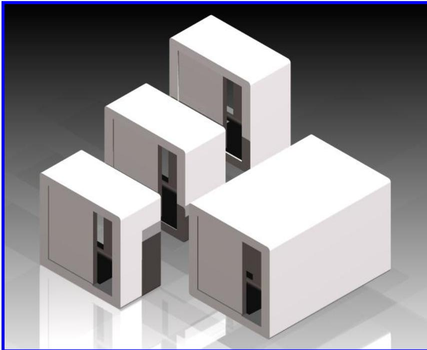
Light trapping connector between ion pump and experimental chamber. Unit is comprised of three, bonded together sub units that have blackened interiors and staggered openings to help stop radiation of various kinds from reaching the experimental unit from the ion pump.
