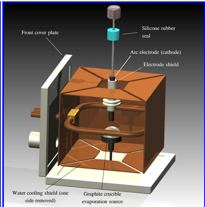
Inside view of vacuum pump showing water cooled shield and evaporated material source.
