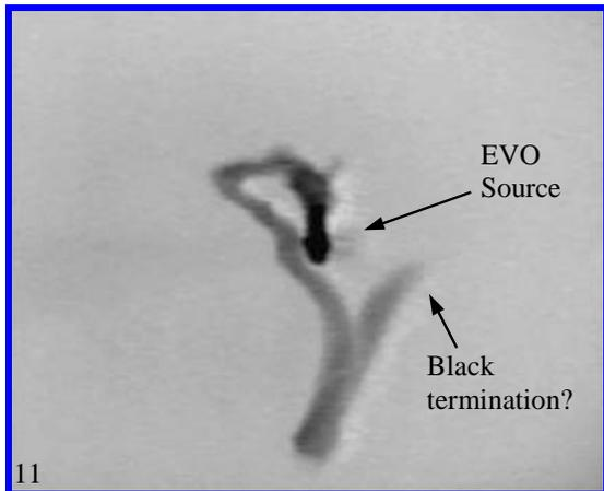
Photo 10 shows an EVO path that is essentially confined to a plane near its source, as indicated by its more or less constant diameter. Photo 11 is similar to Photo 10 but having more extended excursions and a clear but unknown termination.
