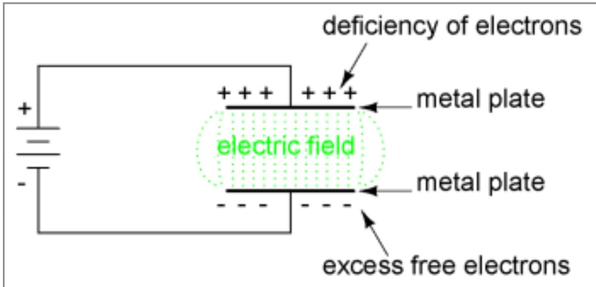
In the previous picture the electric field is shown in green. Notice how the edges are bowed out? This will become very important in the Capacitance Theory of Gravity. This distortion in the electric field is called a fringe effect. It's not very strong compared to the rest of the field. Nonetheless, it is always present on the edge of a capacitor.
