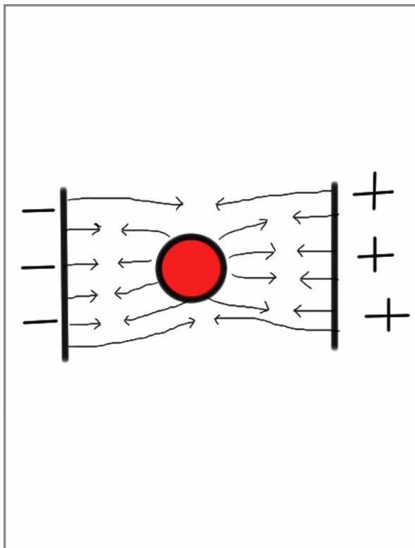
Now we put an object in between the plates. This object has dielectric properties that inhibit the flow of electricity yet enhance the lines of force. This object is electrically neutral. Yet, when it's in the electric field, it is pulled toward both plates equally.
