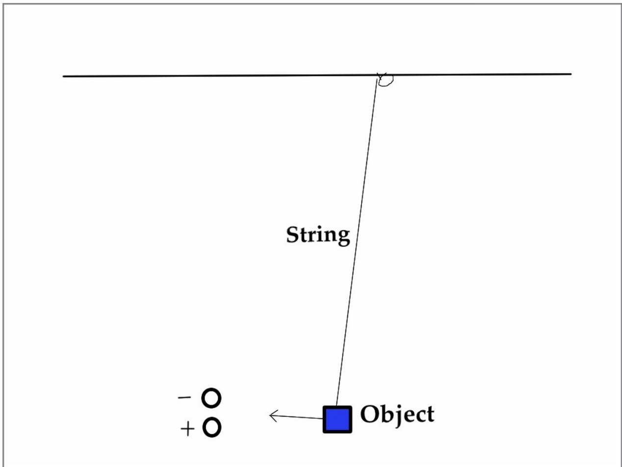
If you use a constant voltage, you need to use a voltage of around 10,000 volts for this to be readily apparent. However, 60 Hz AC, coming right out of the wall, works just as well. It doesn't matter which terminal is charged, so long as they are opposite.
