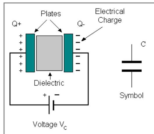
A capacitor is something that is designed to hold opposite charges apart. In doing so, the energy, in the form of electrical charge, is stored.
