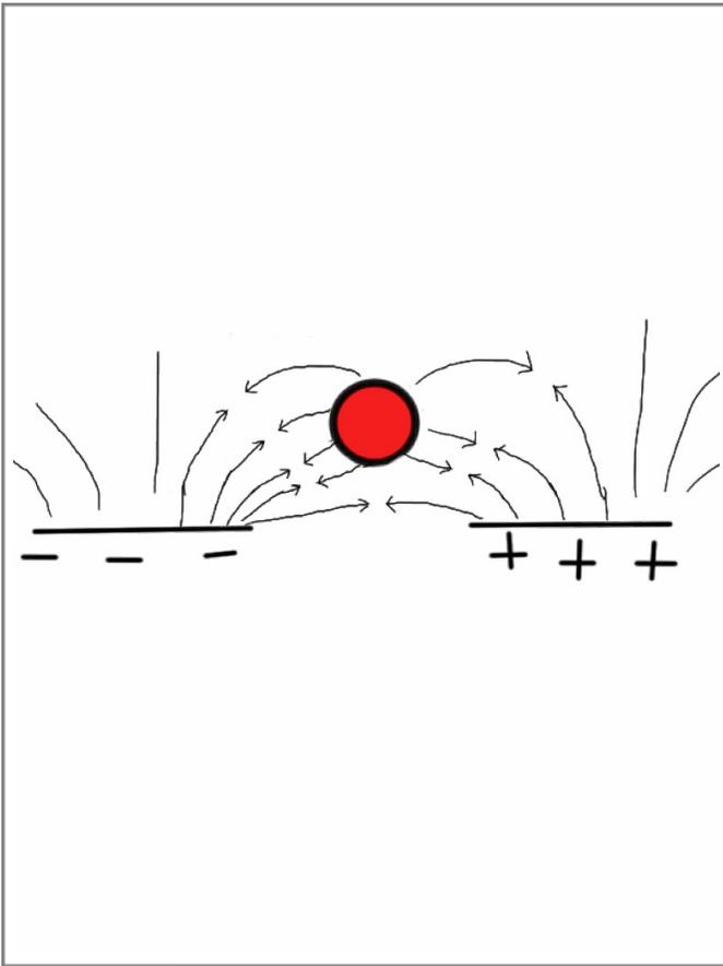
Now we put the two charged plates on their side. There is still an attractive force between them but the electric field is slightly different. The dielectric object still pulls in the attractive lines of force. The plates are also still attracted to each other.
